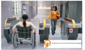
Fare gates accommodate a wide variety of users. Note that the gate assembly is long enough so that exiting passengers do not have to slow or stop walking in order for the gate to open. The gate has multiple smart card targets to speed fare collection. Nanakuma line, Japan
